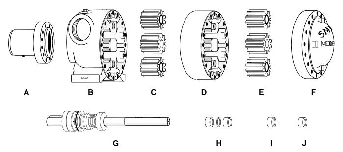
This drawing is made to show the general positions of parts in Smith pumps. It is not drawn to scale, as sizes and configurations do vary from one model type to another. The MC-3 model type was used in the above drawing because it is typical of the majority of units actually in service. Contact the factory if there are any questions. See specific assembly views and parts lists for exact information.
