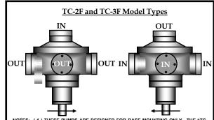
NOTES: (1) THESE PUMPS ARE DESIGNED FOR BASE MOUNTING ONLY. THE "TC-3F" SERIES DO NOT APPEAR EXACTLY AS SHOWN, ABOVE. THEY HAVE A SECONDARY GEAR HOUSING INSTALLED BETWEEN THE GEAR END COVER AND MAIN HOUSING, AND ARE CORRESPONDINGLY GREATER IN LENGTH.
