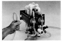
After you finish applying liquid chemical, it is always good practice to flush-out the injector check valves with clean water. To do this, simply remove the suction tube from the chemical container, open the priming valve and let the injector run for about 20 seconds. This flushing procedure will extend the life of the check valves and will enable you to change the injector piston O-ring less frequently.
